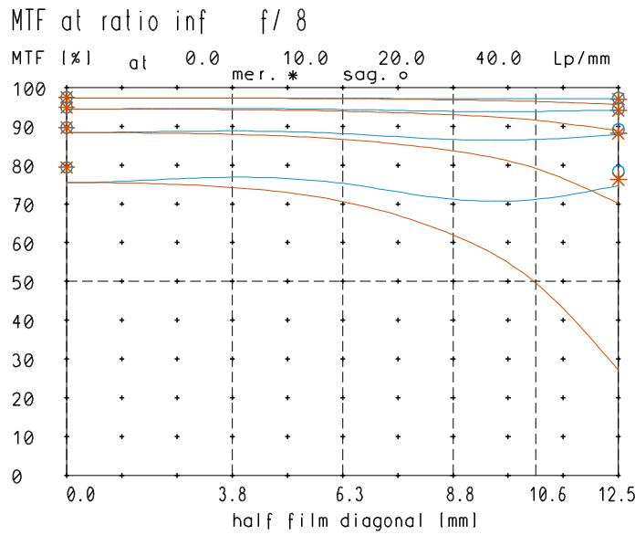
Named frequencies (line pairs/mm) in modular transfer function (MTF) as well as diagrams of relative light fall-off, distortion and longitudinal color aberration refer to film plane.
